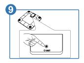
If you would like to change the measurement unit, you can press the button in the battery compartment to cycle through pounds, kilograms or stones.
